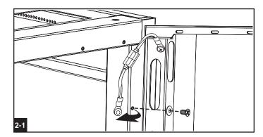
Open the right rear door until it is perpendicular (90 degrees) to the rear of the enclosure, lift it from the hinges and set it aside. Repeat for the left rear door. (If the enclosure is joined to another enclosure, turn the door back toward the enclosure as you lift it from the hinges.)
